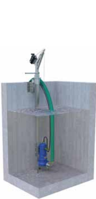
Vertical pole-mounted installation
