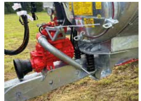
Fitted with Battioni Vacuum Pump
